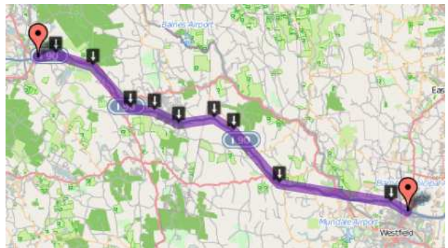
Figure 3: The route between interchanges 2 and 3 of I-90 in Massachusetts after adding “shaping” points to improve the approximation of the road. The distance via shaping points is 30.1 miles.
